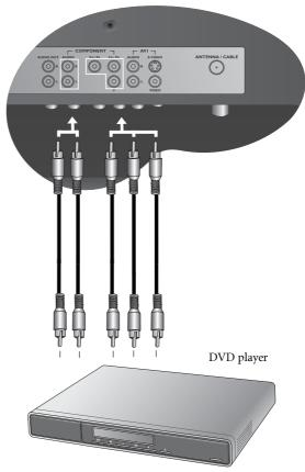
Connect your AV equipment to the TV's Component Y CB/PB CR/PR intput using a Component video cable.
